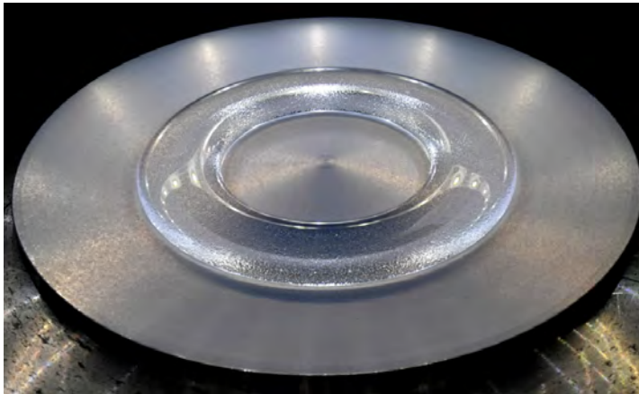
Figure 1. A stable torus of fluid of outer radius R_o = 4.8 cm on a superhydrophobic substrate.
